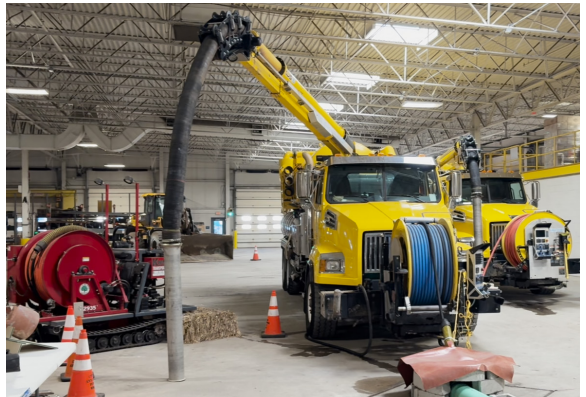
Sanitary sewer equipment and pipe cleaning demonstration and combination sewer cleaning trucks (yellow) and an easement sewer cleaning machine (red)
